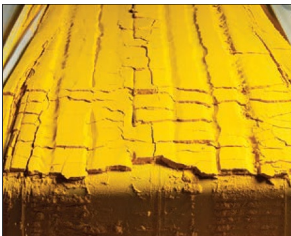
Figure 3.3.1-7. – Yellowcake on the production line
