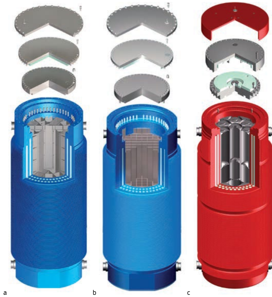
Figure 4.2-3. CASTOR® spent fuel storage casks. (a)V/19 (PWR), (b)V/52 (BWR), (c) HAW28M (HLW).
